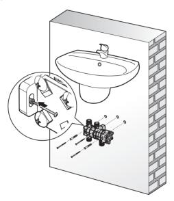
Secure the NaviCirc with the three anchor bolts included with the installation kit.
