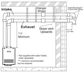
When choosing intake and exhaust terminations, you must use the same type of elbow (i.e. both  $90^\circ$  elbows).
