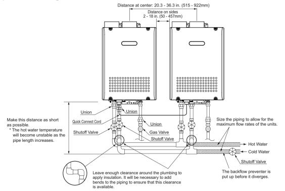
Insulate the hot water piping to prevent heat loss. Insulate and apply heating materials to the cold water supply piping to prevent heat loss and freezing of pipes when exposed to excessively cold temperatures.
