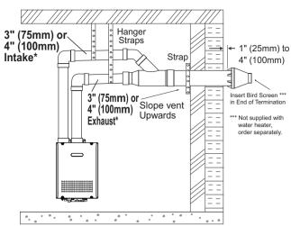
\* 4" (100mm) pipe requires the use of a reducing coupling just prior to the termination.
