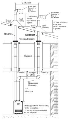
When choosing intake and exhaust terminations, you must use the same type of elbow (i.e. both  $90^{\circ}$  elbows).
